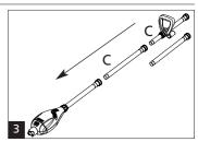
4. The main handle (E) is attached to a tube by simply pushing the narrow end of the handle into the wide end of a tube (C) until tight. Twist and pull the handle to disassemble.
