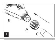
Insert the narrow end of one of the connecting tubes (C) through the opening at the rear of the support handle (D). Position the handle as required and screw the nut (A) until hand tight. It is recommended that the support handle is always located on the tube furthest from the vacuum head.
