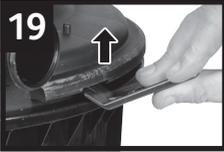
Unlatch the lid clamp (Fig. 2(n)). Gently release and remove the lid by using the 2 levers in opposite slots (Fig. 19). It may help if you remove the attached hoses.
