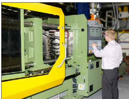
One of the five new injection moulding machines at Hozelock's world-class production facility at Midpoint Park, Birmingham
